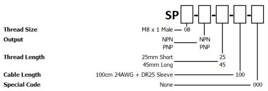
The KA configuration tool is used to specify a standard KA Sensor, other options are available.
